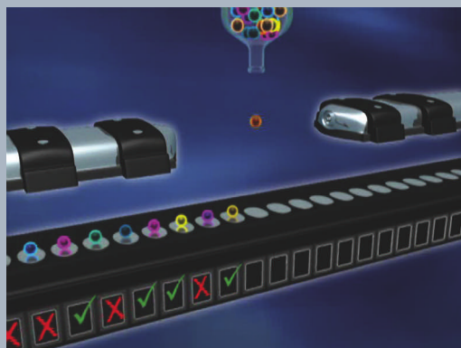
Patient samples are placed in wells on microtiter plates within the Luminex multiplexing instrument, where the sample and bead mixture is excited by lasers. The system's software indicates if a virus is present. Courtesy of Luminex.
